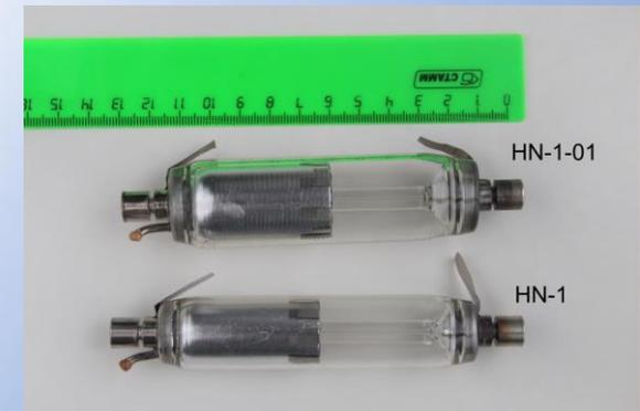
**Helium-Neon laser tubes are widely used for refurbishment of HeNe lasers; interferometry; high-accuracy precision measuring equipment for microelectronics and machinery units.**
